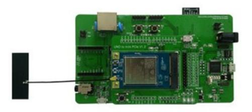
ITM-M487-DK (Azure Develop board) Azure CERTIFIED DEVICE
